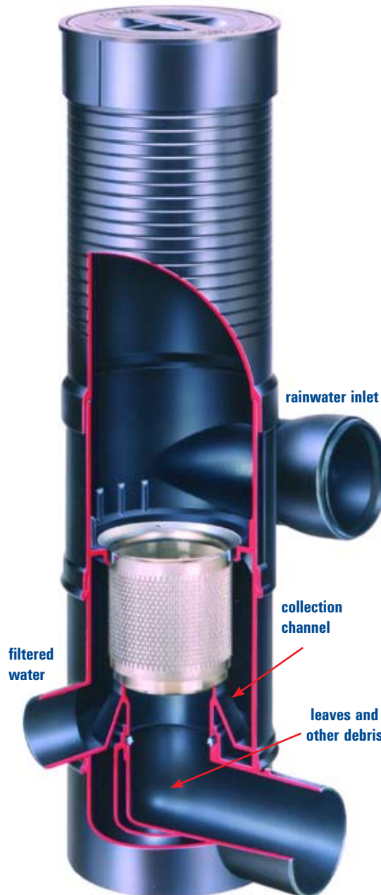
WFF150 vortex filter with extension tube
