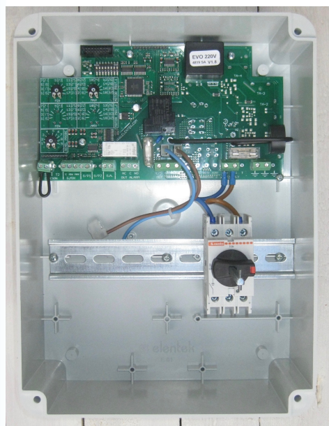
Panel internals with terminal block and DIN rail
