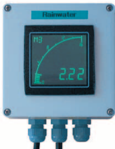
APM meter mounted in plastic box
