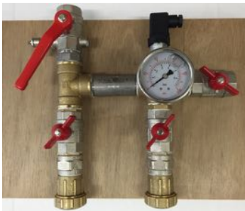
Pump manifold switch-board. Isolating & non-return valves, pressure transmitter, gauge and outlets for expansion vessel.
