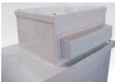
Raised valve housing with screened weir overflow giving a type AB air gap, can be fitted with drop-arm equilibrium float valve or Keraflo valve where required.
