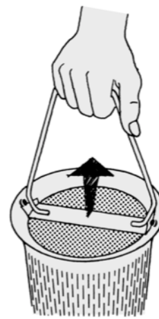
Lift the element clear of the filter body
