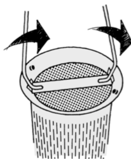
Twist clockwise to locate under the pins
