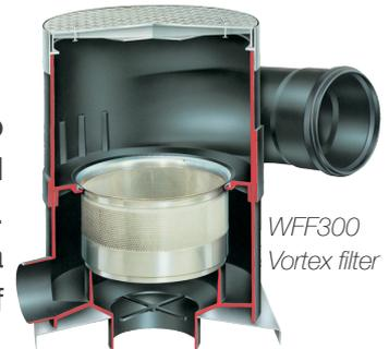
Water is collected from the new barns and an existing adjacent building via a large Vortex filter into a 50,000-litre underground tank. This removes leaves and all other debris larger than 0.38mm. The water is then pumped to an intermediate break tank which is equipped with an automatic back-up from the mains water supply. From here the water is then pumped to several drinking troughs via fine sediment filters and an Ultra-Violet disinfection unit.
